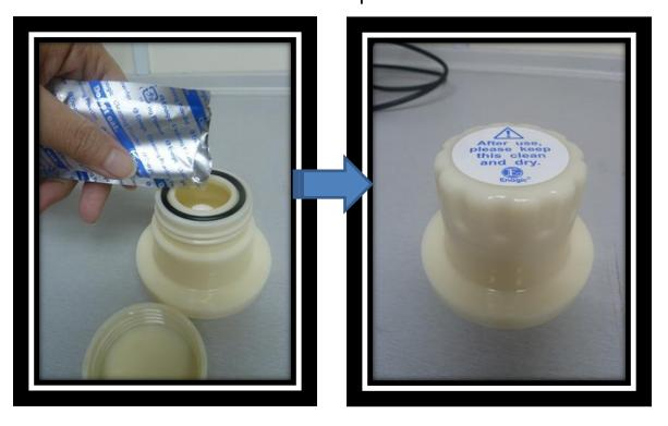
5) Place the CPU (cleaning powder unit) in the machine where the filter was.
