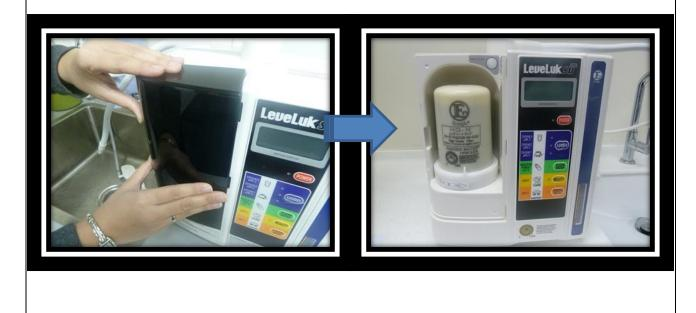
3) Remove the filter from the machine.
