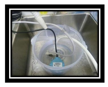
11) Power on the pump. Let the water running for 30 minutes to one hours (depends on the water quality)
