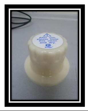
5) Place the CPU (cleaning powder unit) in the machine where the filter was.
