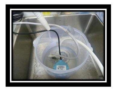
11) Power on the pump. Let the water running for 30 minutes to one hours (depends on the water quality)
