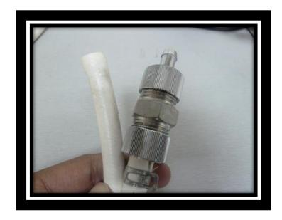
14) Connect white hose to tap water. Then rinse the machine by running water for 5 - 10 minutes with the CPU still in place. (DO NOT TURN ON THE MACHINE YET!)
